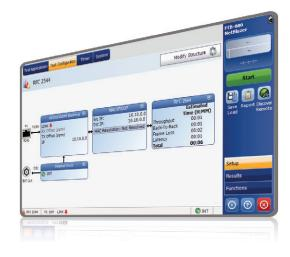
The control panel has icons to access the most important testing elements, buttons for the Setup, Results and Functions screens, as well as a clear pass/fail indicator. Field techs have the assurance that their testing time is optimized.
